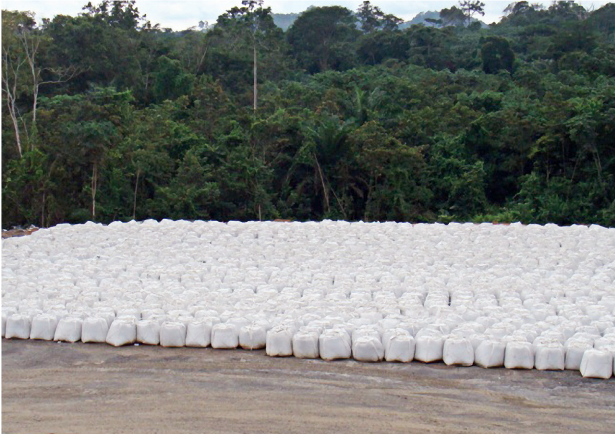
Bitumen Bags storage at a Hot Mix Asphalt Plant, Equatorial Guinea
