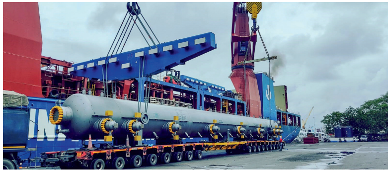
▲ The hydrolyzers are loaded for sea transport in Mumbai, India. ▶ Plant site before modernization. ▼ Plant site after modernization.
